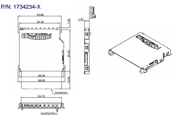
Full Size Connector: Top Mount, Push/Push Insertion/Removal
