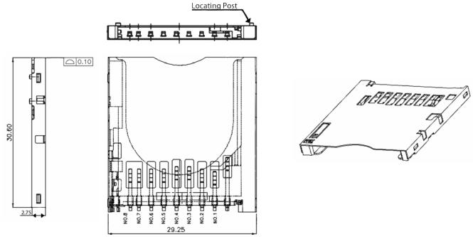
Mini Connector: Bottom Mount, Push/Push Insertion/Removal
